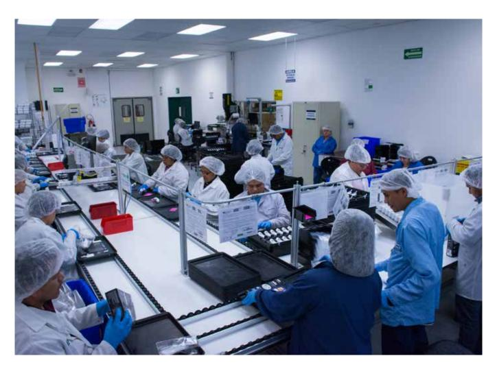
That new facility in Da Nang, Vietnam is 133,000 square feet and currently contains one surface-mount technology (SMT) line to produce electronic circuits. In the future, the facility can be expanded to three SMT lines and multiple final assembly lines without any further construction. Amazingly, it was completed within eight months of site selection.
